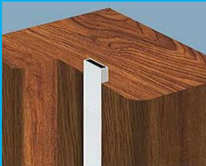
Intumescent heat seal fitted on to the door frame – because there are no cold smoke seals it is permissible to paint over the heat seal with up to 5 coats of oil based paint or varnish
