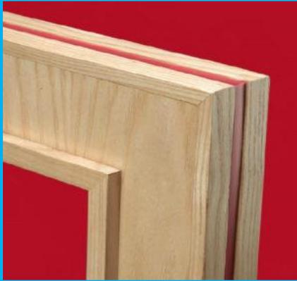
Intumescent heat seal fitted on to the edges of the door – because there are no cold smoke seals it is permissible to paint over the heat seals with up to 5 coats of oil based paint or varnish
