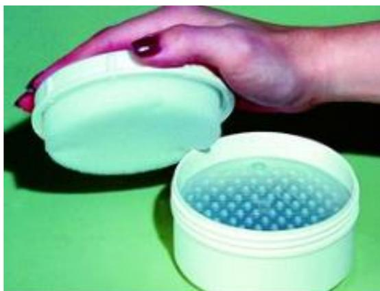
***A typical mercury collector (Whilst using the kit the user must wear gloves)***
