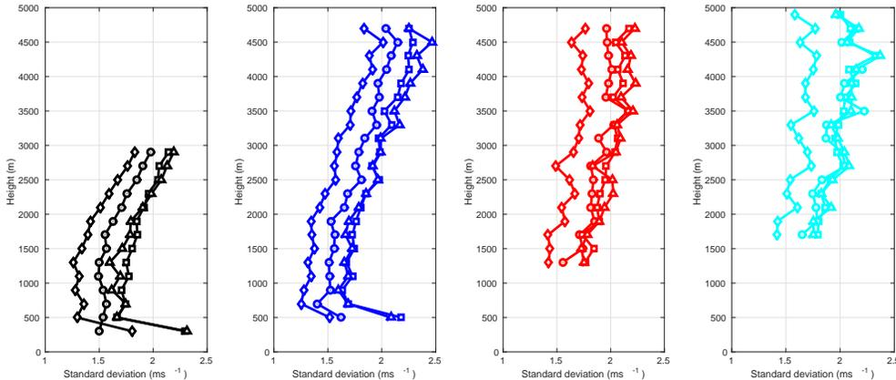
**Figure 4** – Horizontal observation error standard deviation for elevations  $1^\circ$  (black),  $2^\circ$  (blue),  $4^\circ$  (red) and,  $6^\circ$  (cyan) for Case 1 (Control, squares), Case 2 (Alternate background error statistics, diamonds), Case 3 (Thinned raw data, triangles) and Case 4 (New observation operator, circles).
