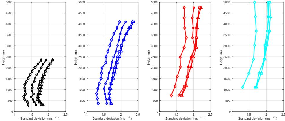
**Figure 8** – Along-beam observation error standard deviation for elevations  $1^\circ$  (black),  $2^\circ$  (blue),  $4^\circ$  (red) and,  $6^\circ$  (cyan) for Case 1 (Control, squares), Case 2 (Alternate background error statistics, diamonds), Case 3 (Thinned raw data, triangles) and Case 4 (New observation operator, circles).
