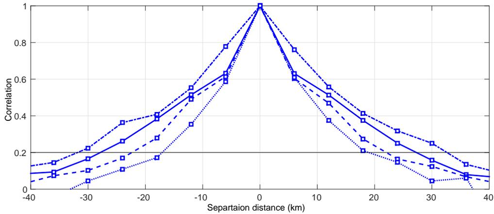
**Figure 5** – Horizontal observation correlations for elevation  $2^\circ$  at height 1.1km (dot), 2.7km (dash), 3.5km (solid) and 4.3km (dot-dash) for Case 1 (control). Error correlations are deemed to be insignificant below the horizontal line at 0.2.
