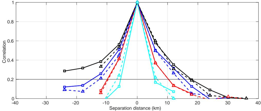
**Figure 11** – Correlations along the beam at range 40km for elevations and approximate heights  $1^\circ \approx 0.8\text{km}$  (black),  $2^\circ \approx 1.5\text{km}$  (blue),  $4^\circ \approx 3.0\text{km}$  (red) and  $6^\circ \approx 4.3\text{km}$  (cyan) for superobbed data (solid lines) and thinned raw data (dashed lines). Error correlations are deemed to be insignificant below the horizontal line at 0.2.
