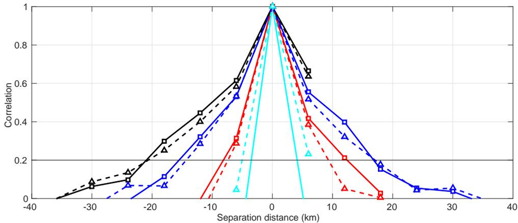
**Figure 10** – Correlations along the beam at height 2.5km for elevations and approximate ranges  $1^\circ \approx 100\text{km}$  (black),  $2^\circ \approx 64\text{km}$  (blue),  $4^\circ \approx 35\text{km}$  (red) and  $6^\circ \approx 22\text{km}$  (cyan) for superobbed data (squares/solid lines) and thinned raw data (triangles/dashed lines). Error correlations are deemed to be insignificant below the horizontal line at 0.2.
