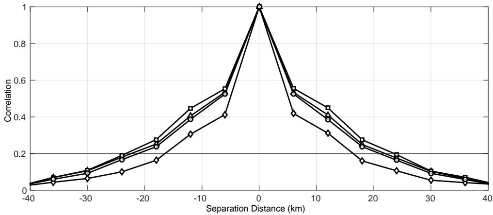
**Figure 3** – All elevation horizontal observation error correlations for Case 1 (Control, squares), Case 2 (Alternate background error statistics, diamonds), Case 3 (Thinned raw data, triangles) and Case 4 (New observation operator, circles) . Error correlations are deemed to be insignificant below the horizontal line at 0.2.
