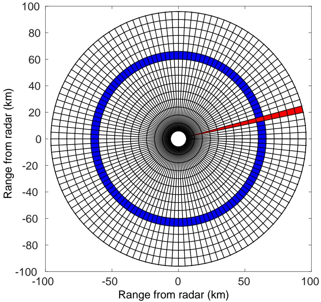
**Figure 1** – A typical radar scan where each box is the location of a superobservation. The blue cells show a group of observations, all at the same height, that would be compared to calculate horizontal correlations. The red cells show observations that would be compared to calculate the along-beam correlations.
