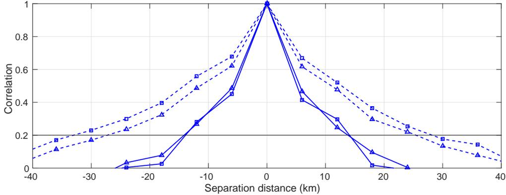
**Figure 12** – Horizontal observation correlations for elevation  $2^\circ$  at a range of 24km (solid) and 90km (dash) for Case 1 (control, squares) and Case 3 (Thinned raw data, triangles). Error correlations are deemed to be insignificant below the horizontal line at 0.2.
