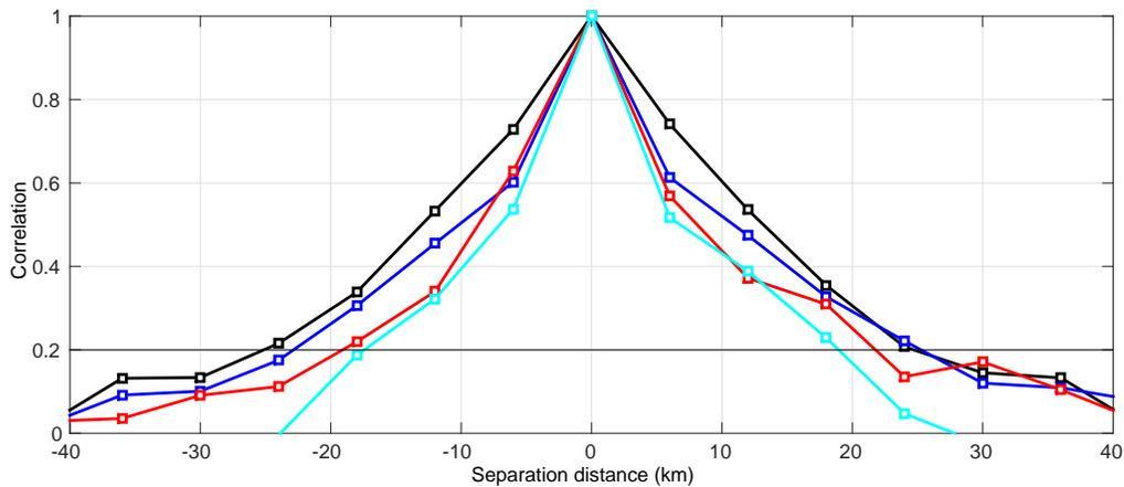
**Figure 6** – Horizontal correlations at height 2.5km for elevations  $1^\circ$  (black),  $2^\circ$  (blue),  $4^\circ$  (red) and,  $6^\circ$  (cyan) for Case 1 (Control). Error correlations are deemed to be insignificant below the horizontal line at 0.2.
