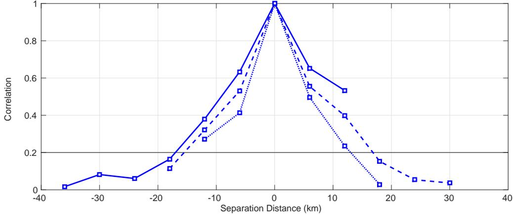
**Figure 9** – Along-Beam observation correlations for elevation  $2^\circ$  at height 1.1km (dotted line), 3.0km (dashed line) and 3.5km (solid line) for Case 1 (Control).
