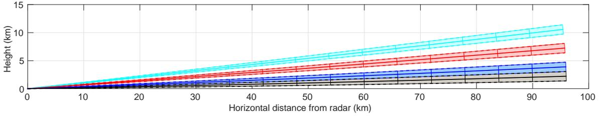
**Figure 2** – A typical radar beam at elevations  $1^\circ$  (black),  $2^\circ$  (blue),  $4^\circ$  (red) and  $6^\circ$  (cyan).
