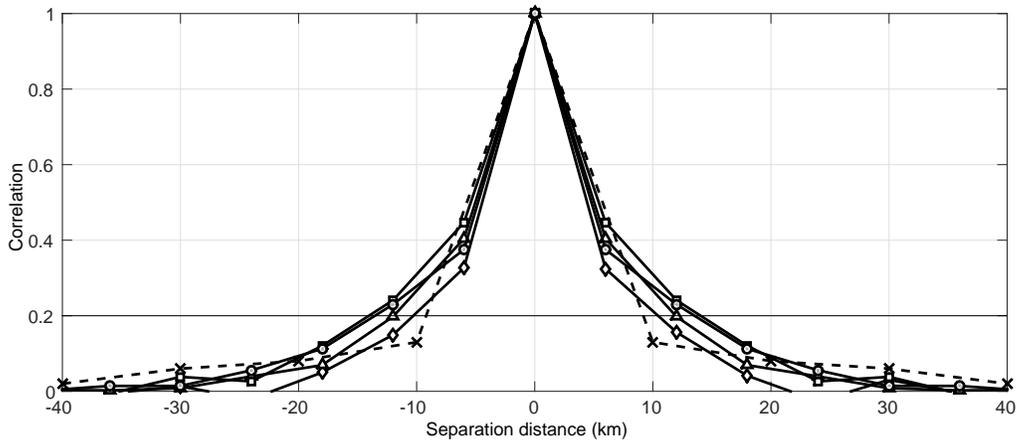
**Figure 7** – All elevation along-beam observation error correlation for Cases 1 (Control, squares), 2 (Alternate background error statistics, diamonds), 3 (Thinned raw data, triangles) and 4 (New observation operator, circles) and those found previously by Météo-France (crosses). Error correlations are deemed to be insignificant below the horizontal line at 0.2.
