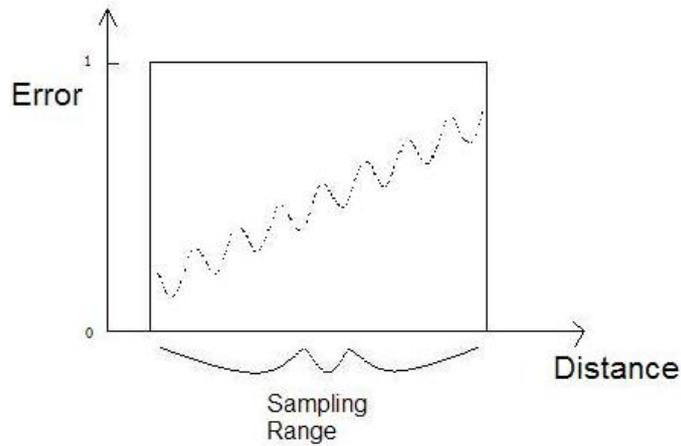
Figure 2.9: Diagram showing the square window multiplied by the sample data
