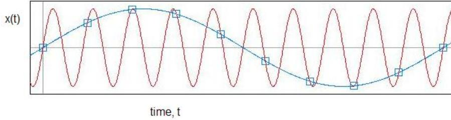
Figure 2.1: Diagram to illustrate the problems with the Nyquist frequency, from [6]
