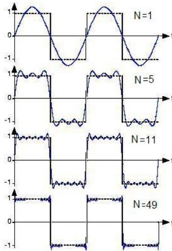
Figure 2.7: Fourier series approximation to a square wave discontinuity, using number of sampling points,  $N = 1, 5, 11, 49$ , [4]
