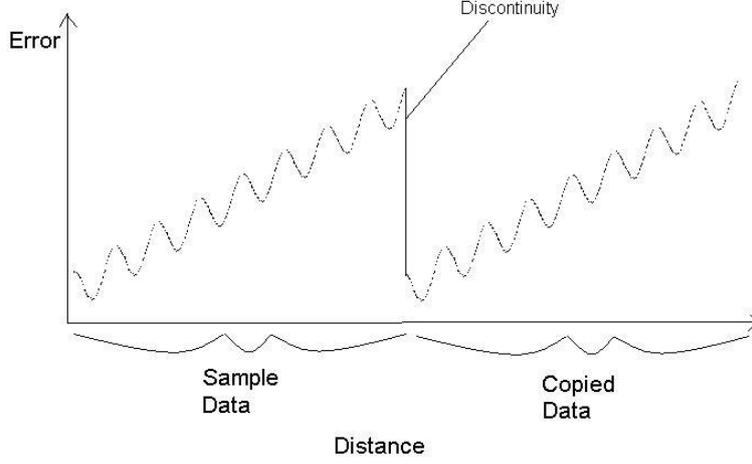
Figure 2.6: Diagram showing a discontinuity forming due to the FFT
