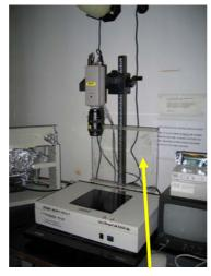
UV transilluminator with shield installed in wrong position, providing the operator with no protection
