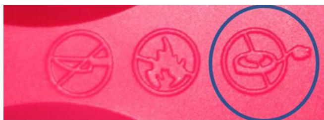
Figure 1. Symbols directly printed in the mould
