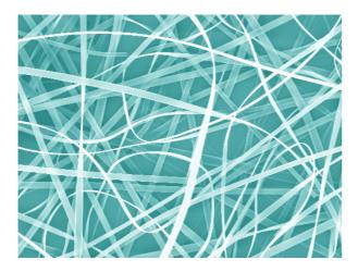
Electrospinning provides an effective route to the preparation of nano and micro fibres of synthetic and biological polymers. It is an enabling technology with applications in medical, pharmaceutical, chemical, textile, electronic industries. The technique produces very fine, nano to micrometer diameter, fibres in random matts as shown above or in more controlled structures.
