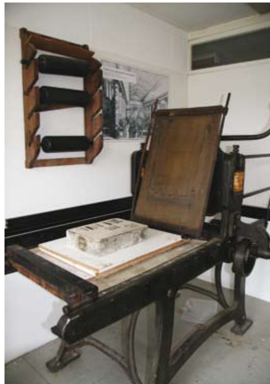
Lithographic press with lithographic stone
