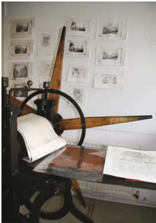
Intaglio press with copperplate and prints and ink rollers
