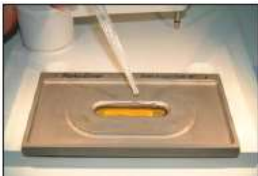
Figure 4. ATR analysis of a liquid sample.
