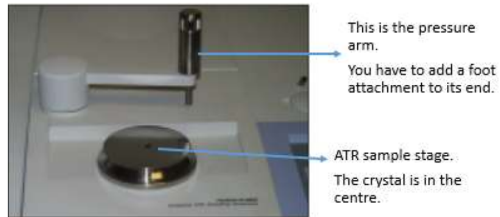
Figure 1. Sample stage in a FTIR-ATR.
