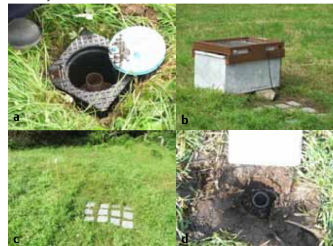
Figure 3 a) TDR access tube b) remote sensing data logger disguised within a modified cattle trough c) metal protective plates covering the monitoring equipment d) piezometer tube (cap removed) used to monitor water table depth and collect samples for chemical analysis
