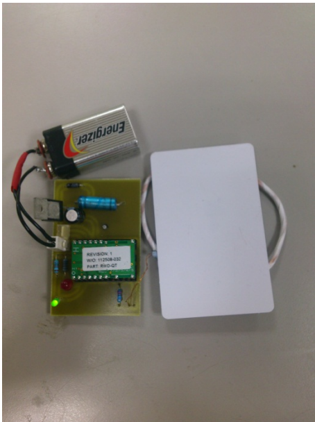
Figure 1. The RFID board with an RFID tag
