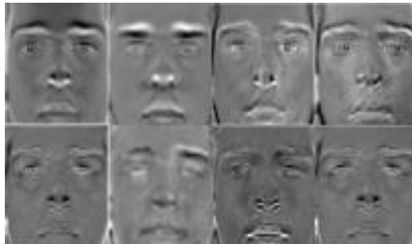
Figure 2. Constructed Eigen Faces from PCA of image set
