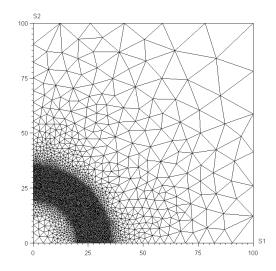
Figure 4.5 - Unstructured mesh use to discretized the Black-Scholes PDE, with knock out barrier set between £20 and £35 (generated with Gmsh (http://www.geuz.org/gmsh/)
