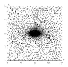
Figure 4.6 - Unstructured mesh use to discretized the Black-Scholes PDE with elliptical barrier imposed on the option (generated with Gmsh (http://www.geuz.org/gmsh/)
