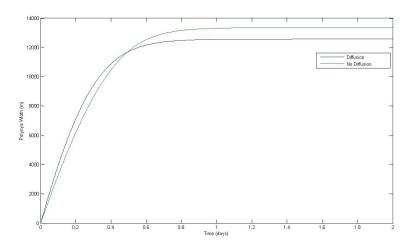
Figure 4.7: Comparative opening phase for a polynya with and without the ice diffusion included in the parameterisation, wind speed is  $20ms^{-1}$
