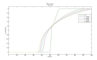
Figure 4.4: Diffusion in a 2m slab of pack ice with a parabolic front
