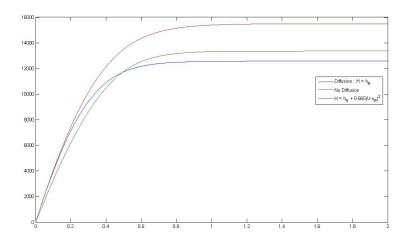
Figure 5.5: Comparative opening phase for a polynya with and without the altered boundary condition, wind speed is  $20ms^{-1}$
