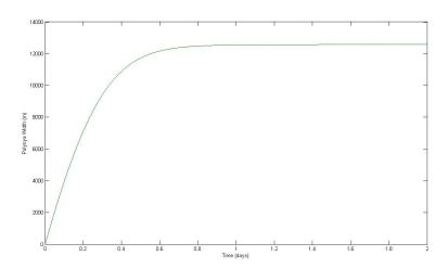
Figure 4.6: Polynya opening with diffusion in the pack ice, wind speed is  $20ms^{-1}$
