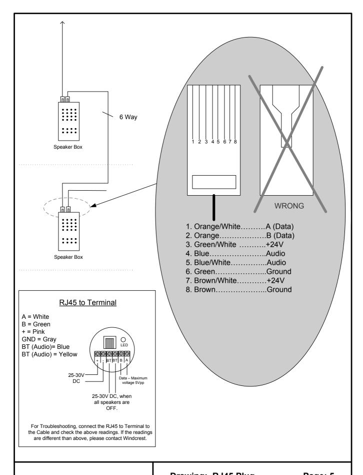
RJ45 Plug & RJ45 Plug to **Terminal**
