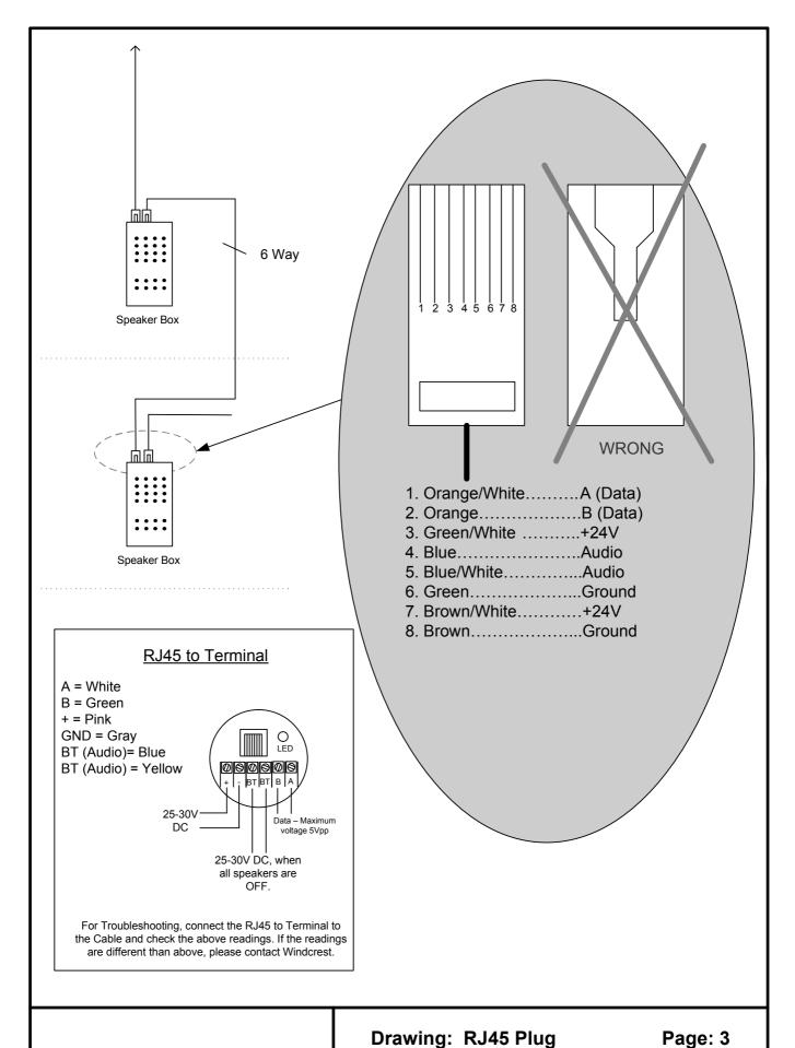
RJ45 Plug & RJ45 Plug to **Terminal**
