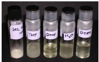
**Figure 3** Solid gel (100 mg) obtained at a Diazirine:MePEO<sub>5000</sub> mole ratio of 2:1 and gel swollen in THF (125 mg mL<sup>-1</sup>), dimethylformamide (125 mg mL<sup>-1</sup>), water (110 mg mL<sup>-1</sup>) and dichloromethane (90 mg mL<sup>-1</sup>)
